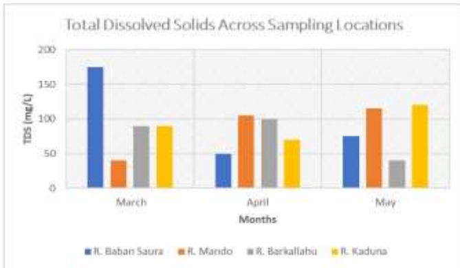
Figure 7. Variation in total dissolved solids of sampling rivers within the sampling period
