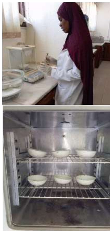
Fig. 1. Weighing and drying samples in the oven at 105 °C (Author, 2024).
