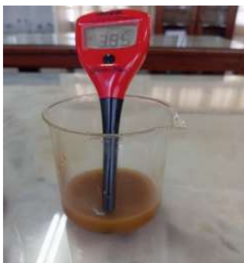
Fig. 3. Direct potentiometric pH reading in samples (Author, 2024)
