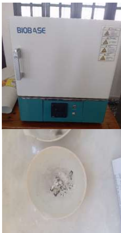
Fig. 2. Muffle furnace, device used to incinerate samples for subsequent quantification of ash (Author, 2024).
